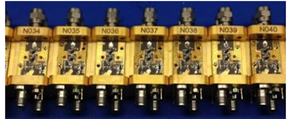
Fig. 20. LNA carriers open side: Pol-A, opposite side: Pol-B. Connectors provide DC bias, lines for voltage monitoring, and 3 RF ports for Pol-A, Pol-B, and noise injection.
