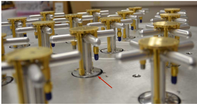
Fig. 9. Dipole array over the ground plane. Arrow highlights thermal gap between dipoles and ground plane.
